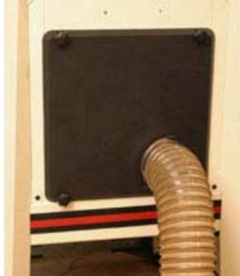
Locating the motor fully within the cabinet (left) allowed us to add effective dust collection in the form of a special cabinet floor and this rear cover (right) featuring a molded in 4" hose connection.
